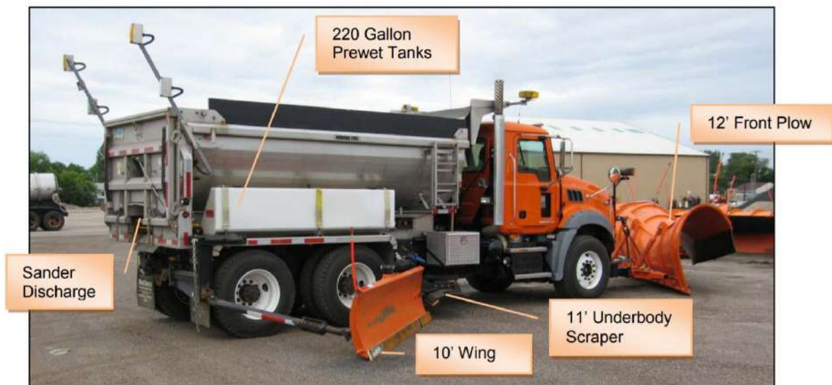
Above: A typical plow will have a 8-12' front plow but can include an additional wing. Plowing 180 miles of County Highways for the general public requires trucks that do this quickly and effectively.
