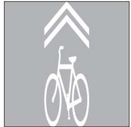
Shared lane marking MUTCD Fig. 9C-9
