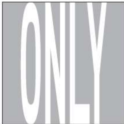
Pavement marking MUTCD Fig. 9C-5
